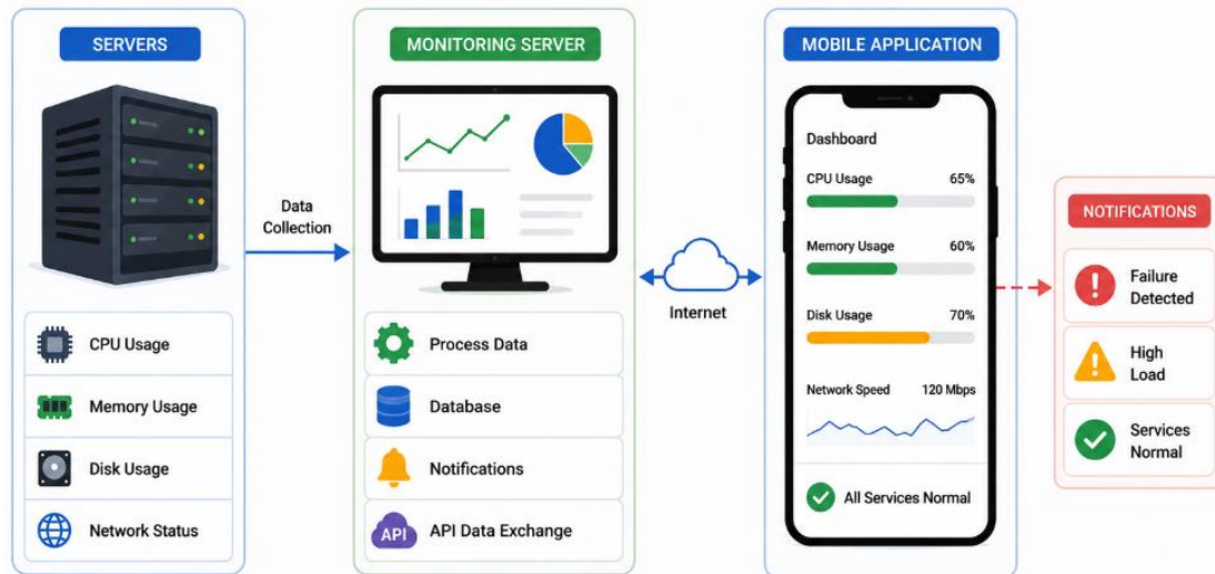
Figure 1. Architecture of the Mobile-Based Server Monitoring System
